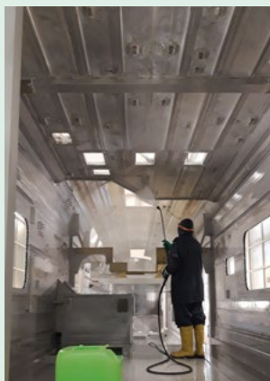
Pre-painting degreasing treatment using a VOC-free solvent.
